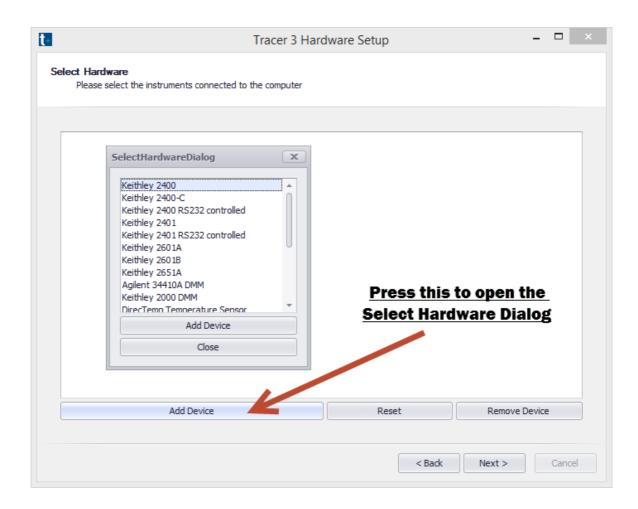
In this part of the wizard the system components are defined. Everything you have connected to the computer has to be indicated here. This means Keithleys, Pt100 sensors, DMM's, Relays, etc...
