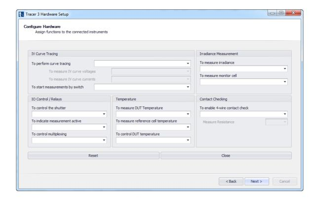
In this last screen the functionality of the defined instruments is configured. Any device can support one or more functions. For example you can use a Keithley 2400 SourceMeter to measure the IV curve of a solar cell, but it can also be used to control the shutter of a solar simulator. The Keithley 2400 has an IO connector on the back that can provide this functionality.
